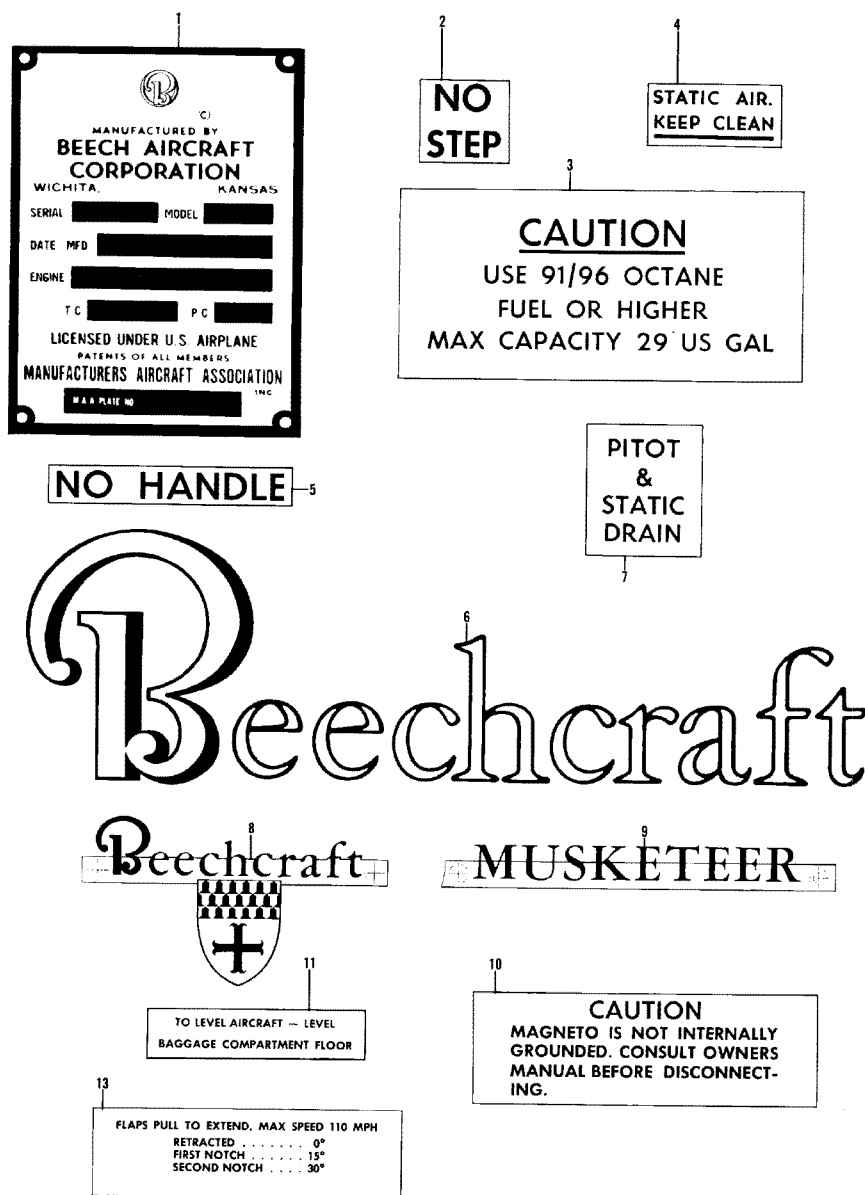
Figure 1. Interior & Exterior Markings (Sheet 1 of 2 Sheets)
